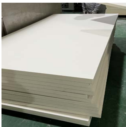
Double sided fiberglass cement tissue +PIR foam
